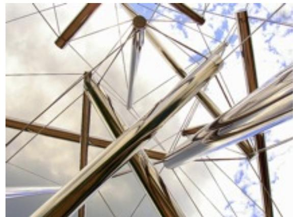
In a tensegrity structure, the beams (compression) are floating in wire (tension). In the human body, the bones (compression) are floating in the fascia (tension).
